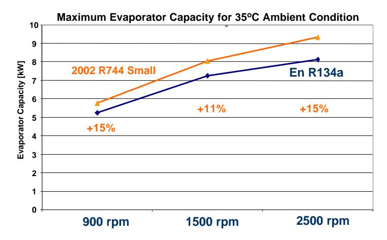
Even with the smaller evaporator, R-744 capacity is superior to En R134a
